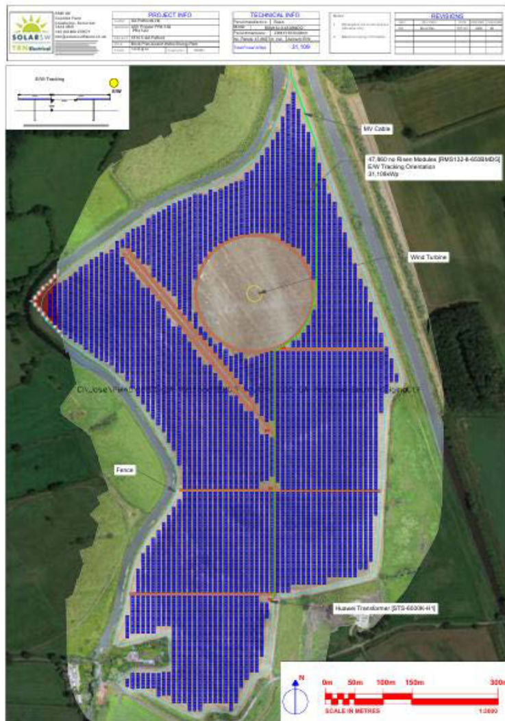
Fig 2 – Initial Concept Arrangement (Maximum) capacity of the Asland Walks Site – single turbine (located centrally) and 27MWp solar arrays. Export to Grid required for surplus Area 35.84ha
