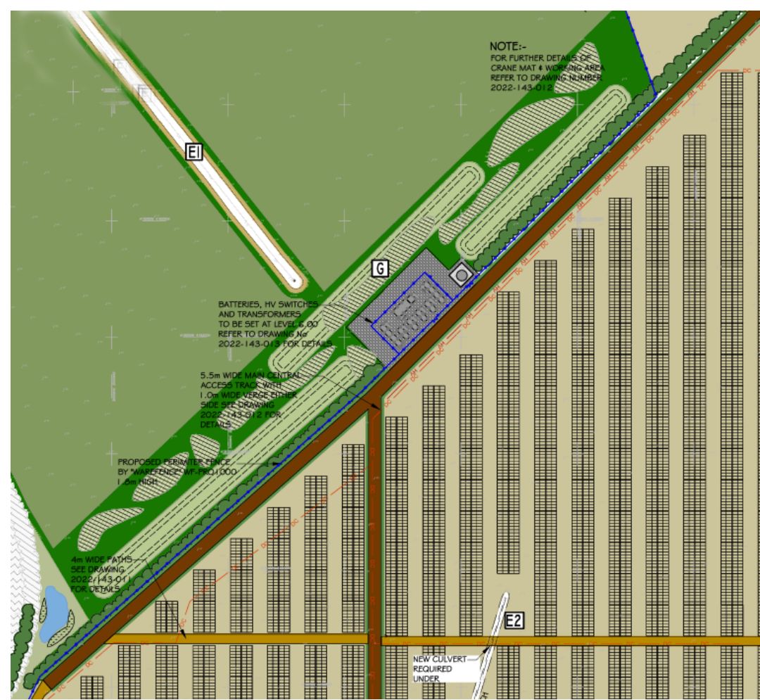
Extract – GSA Dwg 2022-143-011H - General Arrangement to Solar Farm
